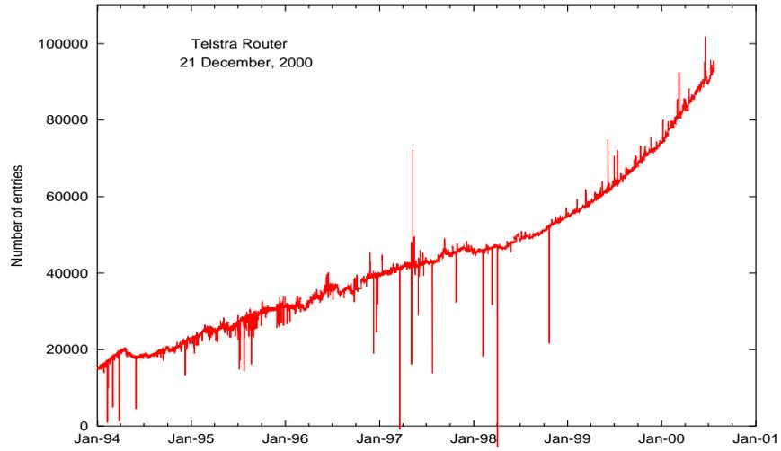
Figure 5: Table growth of a typical backbone router
