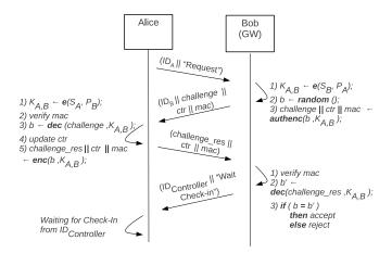
Fig. 3. Detailed handshaking procedure.
