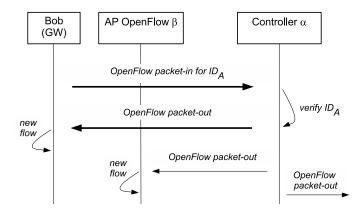
Fig. 5. OpenFlow messages for the new flow.
